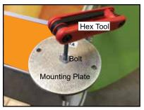
5) Tighten bolt, using hex tool, to secure.
